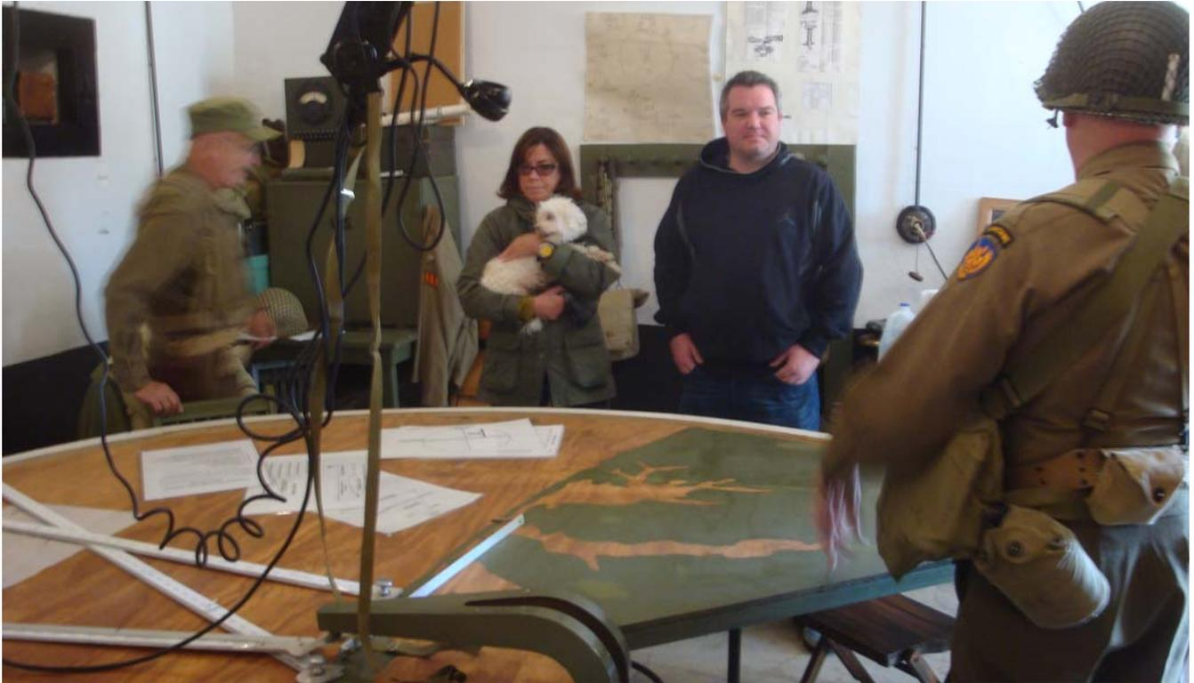
Below, MAJ Winslow explains the plotting board's "gun arm" to the public. The Gun Arm represents the physical line of sight from the seacoast battery itself to the target. By placing this arm on the "plotted point" of the target location, it gives the range, in yards, and azimuth, in degrees of the target to the battery. This 'raw' data tells the Battery which way they need to turn the guns, and how high or low they need to elevate the gun tubes to hit the target.
