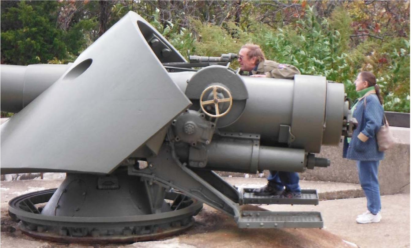
Below, are the ships they are viewing, as seen through the M1904 telescopic gunner's sight. They are an outbound car carrier, and an inbound container ship. This scope, used by the gun pointer, allowed him to physically put "eyes on target".
