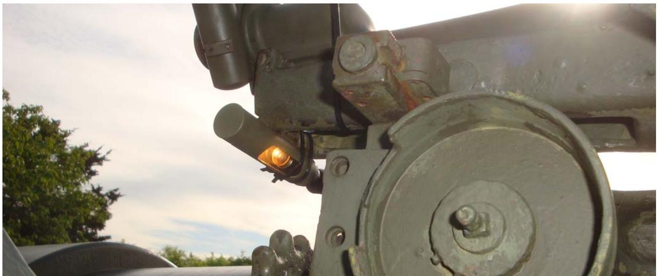
Looking from the gun pointers position, one can see the electric cable for the M1904 sight cradle light and the reticle light on the M1904 telescopic sight. The reticle is the vertical line inside the sight which is used to accurately track a target (in this case ships). This is the first time lights have been on this carriage since 1948, a remarkable milestone in the Battery's restoration.
