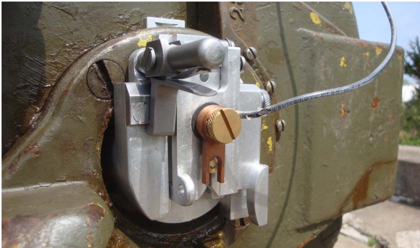
The device below is shown ‘open,’ with the “primer” partially extracted. These are specially produced primers designed to complete an electric circuit. Once we have perfected the reliability of these primers to complete an electric circuit, we will use them to complete a circuit for an audible “boom”. Next step, figuring out the best way to produce that “boom”. Any ideas?
