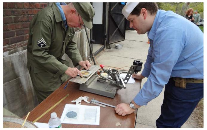
Below is a closer view of the marking machine as T-5 Komorowski sets it up to mark the arm scale. The disk he is centering is the marking guide and is operated with the red handled arm in the center of the photo
