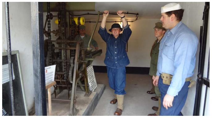
Below, SGT Minton operates the hoist as BM2 Kaiserman moves a shell forward on the shell table to be picked up by the hoist tongs as 2LT Taylor observes from the left. Members ran five shells up the hoist, and found that there was almost no physical change in force needed for cranking the mechanism, which is quite easy to do.
