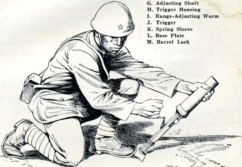
Figure 1.—Japanese Model 89 Grenade Discharger and Ammunition. (The correct position for firing is shown in the bottom view.)
