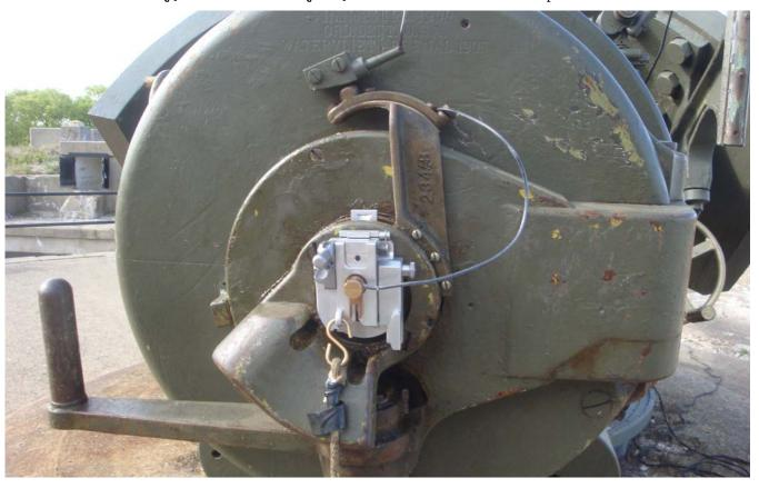
Approximately two years ago, AGFA secured several light fixtures used for fire control instruments in WWII. After locating the correct reproduction electrical plugs (identical to those used on Model T Fords), we fabricated the lights that would have been used on the gun carriage in nighttime or low-light conditions. One is seen here on the elevation drum of Gun No. 1.
