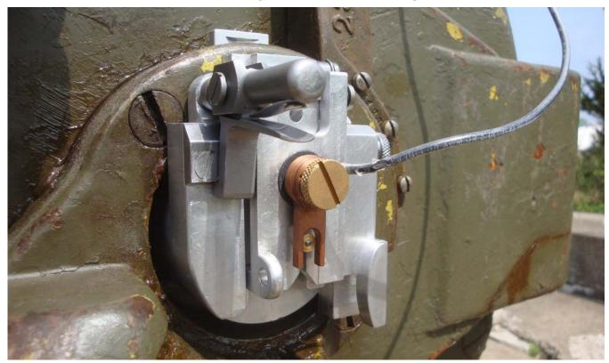
The device below is shown 'open,' with the "primer" partially extracted. These are specially produced primers designed to complete an electric circuit. Once we have perfected the reliably of these primers to complete an electric circuit, we will use them to complete a circuit for an audible "boom". Next step, figuring out the best way to produce that "boom". Any ideas?
