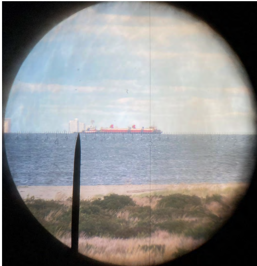
The ship below is being tracked by 2LT Gonzalez using the M1910A1 Azimuth Instrument. The ship is about five miles distant.
