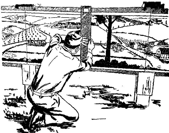
FIGURE 87.—Using target template to divide a vertical target into spaces to give score for distribution.
